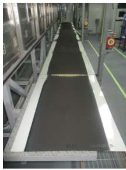
Photo 3: Specimen after the test. (As seen from the exhaust end)
